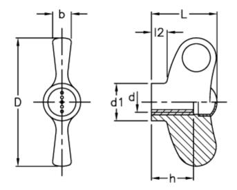
$$\begin{array}{lll} b & = 10 \\ D & = 70 \\ d1 & = 20.0 \\ d \, 6H = M10 \\ h & = 20 \\ L & = 36 \end{array}$$
